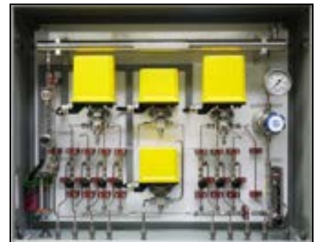
Multiplexed SCS 0-20 ppm H 2 S in 7 streams
