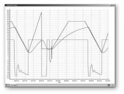
Both data logging and trending are available and the user can trend and view live data, with a scaleable time axis between 1 minute and 1 month. This utility also offers a Historical Review mode and data can be logged onto the PC hard disk, from which it may be retrieved and analysed in an Excel spreadsheet.
